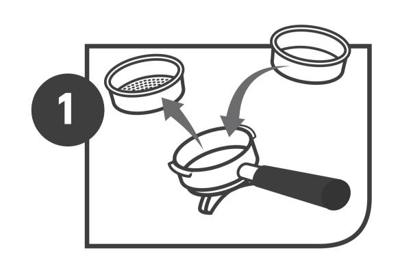
Remove coffee filter from group handle, and replace with "blind" filter or blank basket.
