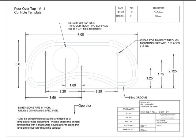
\* If printing a digital copy of the cut-hole template it is important to check a known dimension on the print before use to be certain the template has not been scaled by your printer or printing software.
